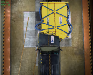
52 working condition (2.27t vehicle) Side impact test
