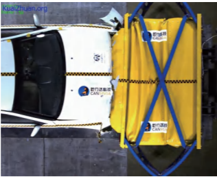
50 working condition (1.1t vehicle) Frontal impact test
